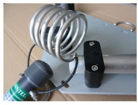
Connect a 1:1 balun to the dipole center (recommended) with two wire jumpers no longer than 8-10 cm (the length affects the resonance of all bands), if you decide not to use the balun, connect terminals of the coaxial opening it as a V directly to the two bolts. Even in this case make sure that the two terminals of the coax does not exceed 10cm. If too long, the antenna will resonate slightly lower. Seal the coax with good quality sealing glues.
